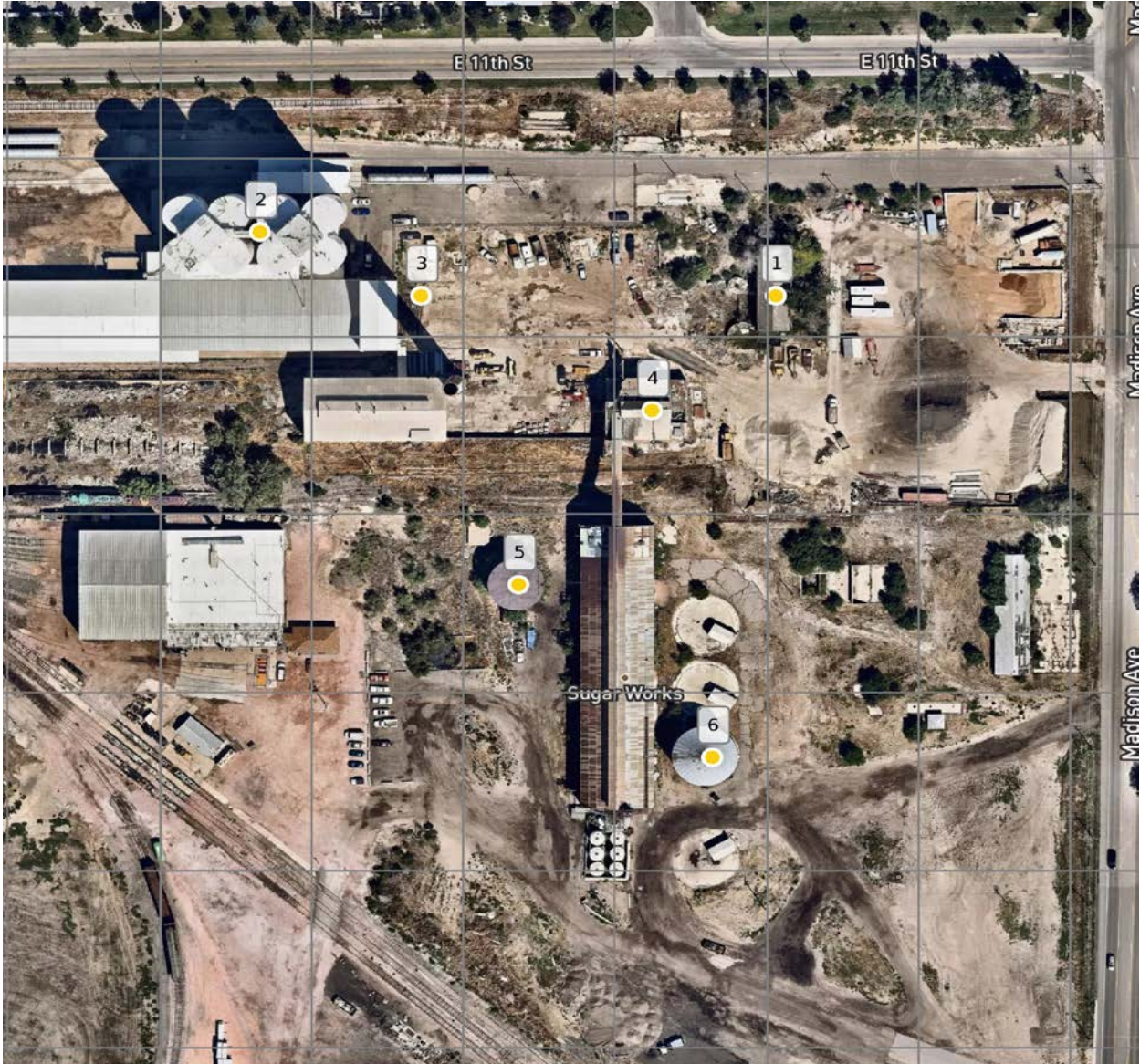
Key: 1. Office Building (described in section 21); 2. Assemblage of eight concrete silos; 3. Concrete smokestack; 4. Building ruins (possibly part of the historic main factory building); 5. Molasses syrup tank; 6. Metal grain bin
