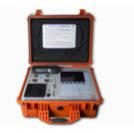
New field test kit for commercial applications. This device tests electric meter accuracy as well as all associated equipment that is used to determine the energy usage.
