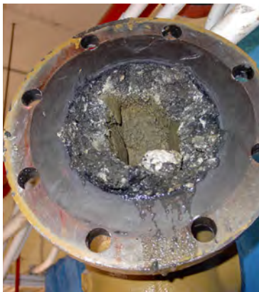
Fats, oil and grease build-up on the interior of a Loveland sewer line.
