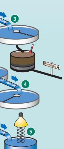
clarification basins. During its 3-hour visit there, more material will settle to the bottom of the tank while lighter material and non-water soluble liquids like cooking oil will float to the top. The bottom sludge moves into the anaerobic digestion tank where it is heated to about 95 degrees and remains for about a month while a biological process digests the organic material. It's then collected, hauled away and used as soil conditioner on farmland.
