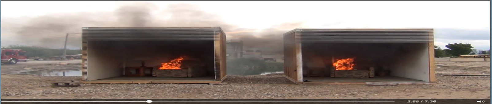
Prior to Fire Sprinkler activation in the right burn cell - 2:55 into demonstration
