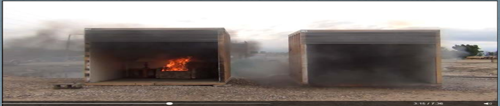
Fire Sprinkler activation in the right burn cell - 3:15 into fire demonstration.
