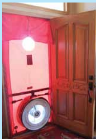
The blower door test helps identify air leaks in the home. Sealing those leaks saves energy and money.
