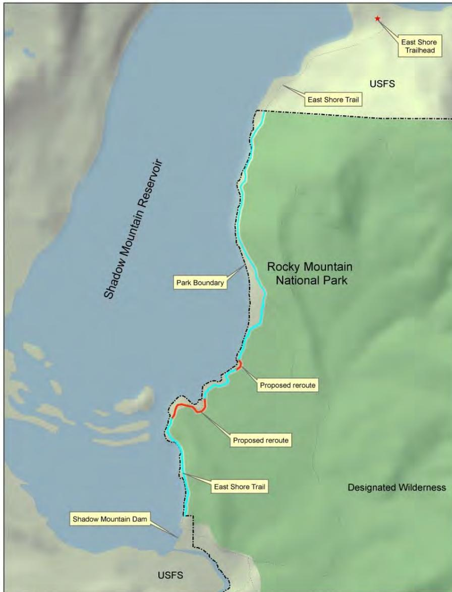
Note: The wilderness boundary is located fifty feet (50') east of the centerline of the proposed alignment of the East Shore Trail. The finished trail must be located a minimum of twenty-five feet (25') west of the wilderness boundary.
