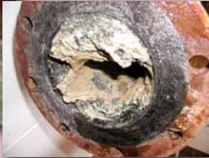
Above: Chunks of grease that arrived at the wastewater treatment plant. Bottom right: Pipe clogged with grease.
