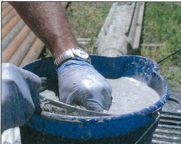
Figure C18. Photograph of removal of mud from cuttings at MW02.
