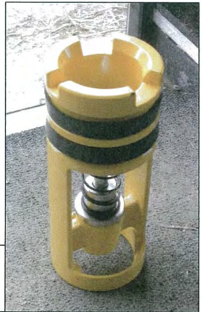
Figure C3. Photograph of blowout preventer for drillstem.
