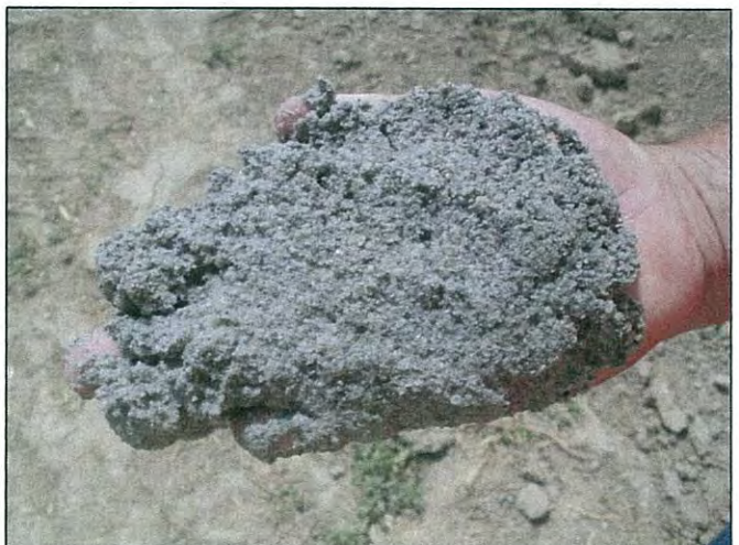
Figure C19. Photograph of white coarse-grained sand targeted by local well drillers and media in which screens are set in for both deep monitoring wells.
